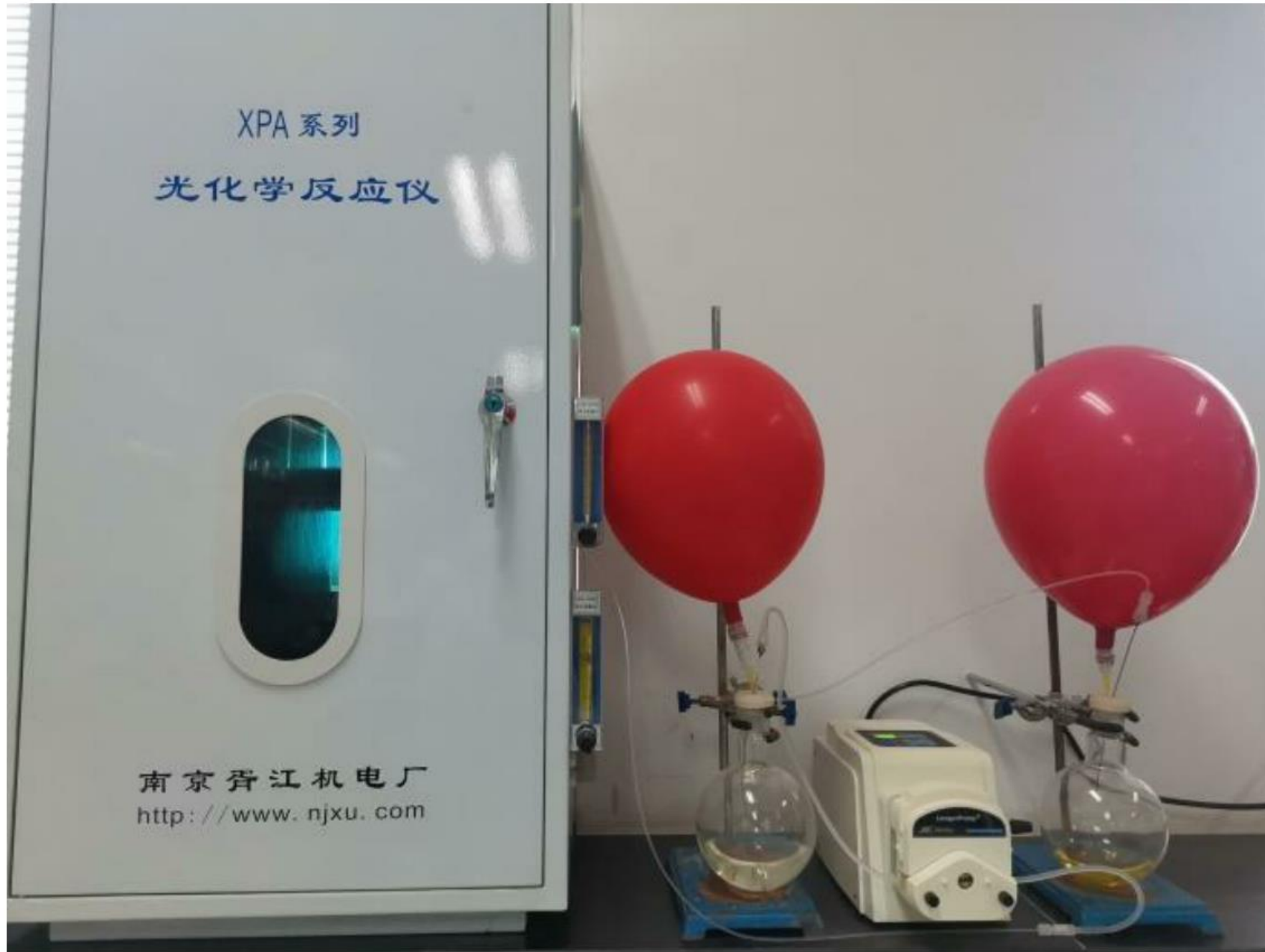
Gram-scale photochemical flow reactor with the peristaltic pump.
